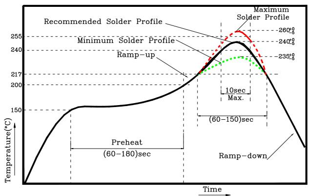
• Reflow soldering should not be done more than two times .
